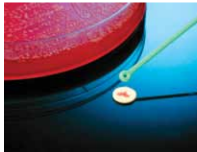
Nitrocef HardyDisks™, Cat. no. Z7301, test for beta-lactamase activity in bacteria.
